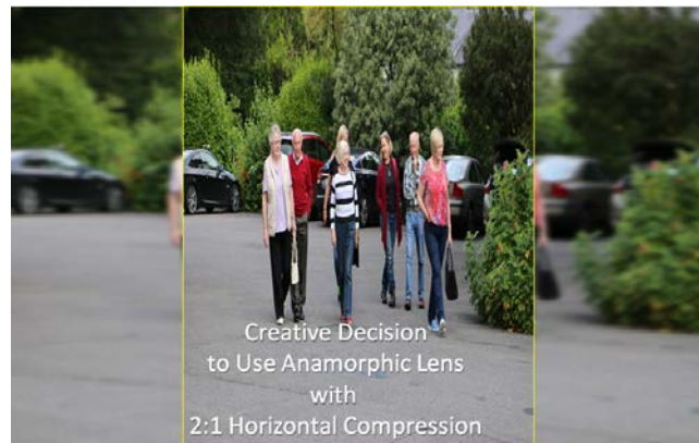
Figure 26 2:1 anamorphic lenses will horizontally compress the image from the lens into the camera
