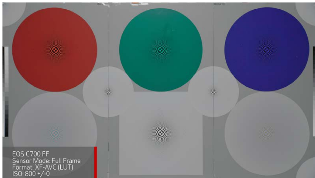
Figure 40 4K Test Chart that facilitates Examination of Luma and Chroma Resolution and Aliasing
