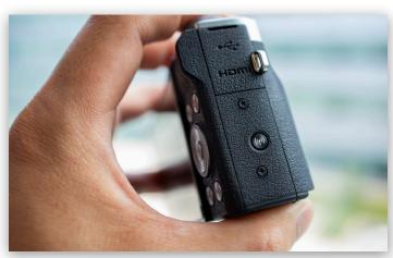
Turn camera on and press Wi-Fi button on the side
