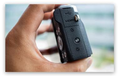
Turn camera on and press Wi-Fi button on the side.
